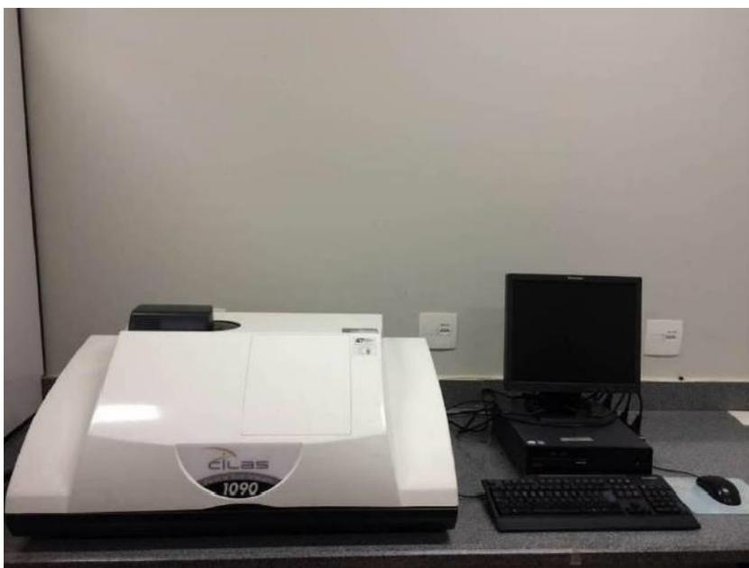
Figura 13- Cilas 1090 *Laser Particle Size Analyzer*.
